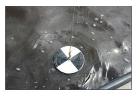
*Figure 3.* Secchi disk being lowered into water to measure clarity. (https://www.flickr.com/photos/usace\_albuquerque/5999717664)
